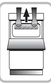
The cooker is designed to fit between kitchen cabinets spaced 500mm apart. The space either side need only be sufficient to allow withdrawal of the cooker for servicing. It can be used with cabinets one side or both as well as in a corner setting. It can also be used freestanding. Adjacent side walls which project above hob level, must not be nearer to the cooker than 150mm and should be protected by heat resistant material. Any overhanging surface or cooker hood should not be nearer than 650mm.
